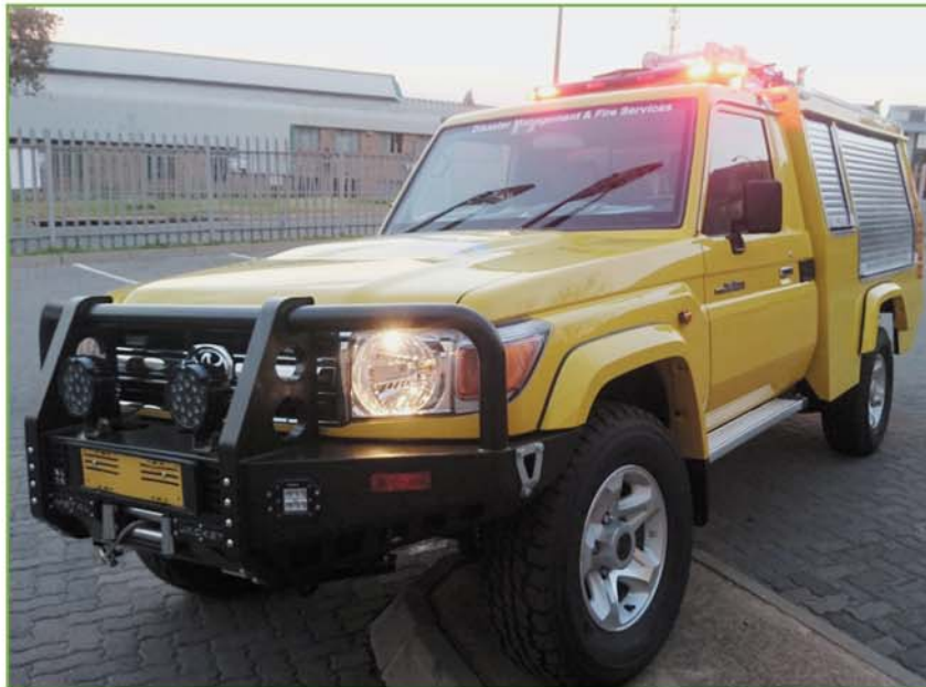
RIV Response Vehicle with UHP fire fighting system, foam making abilities, rescue tools and others.
