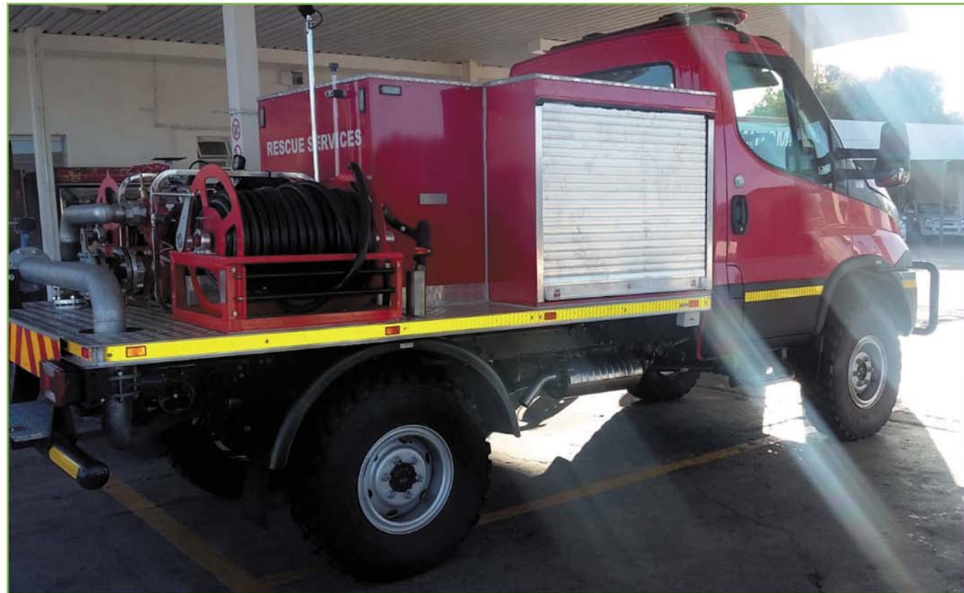
Rapid response vehicle with foam making ability and rescue tools. all built on a Iveco Baily 4 x 4 chassis
